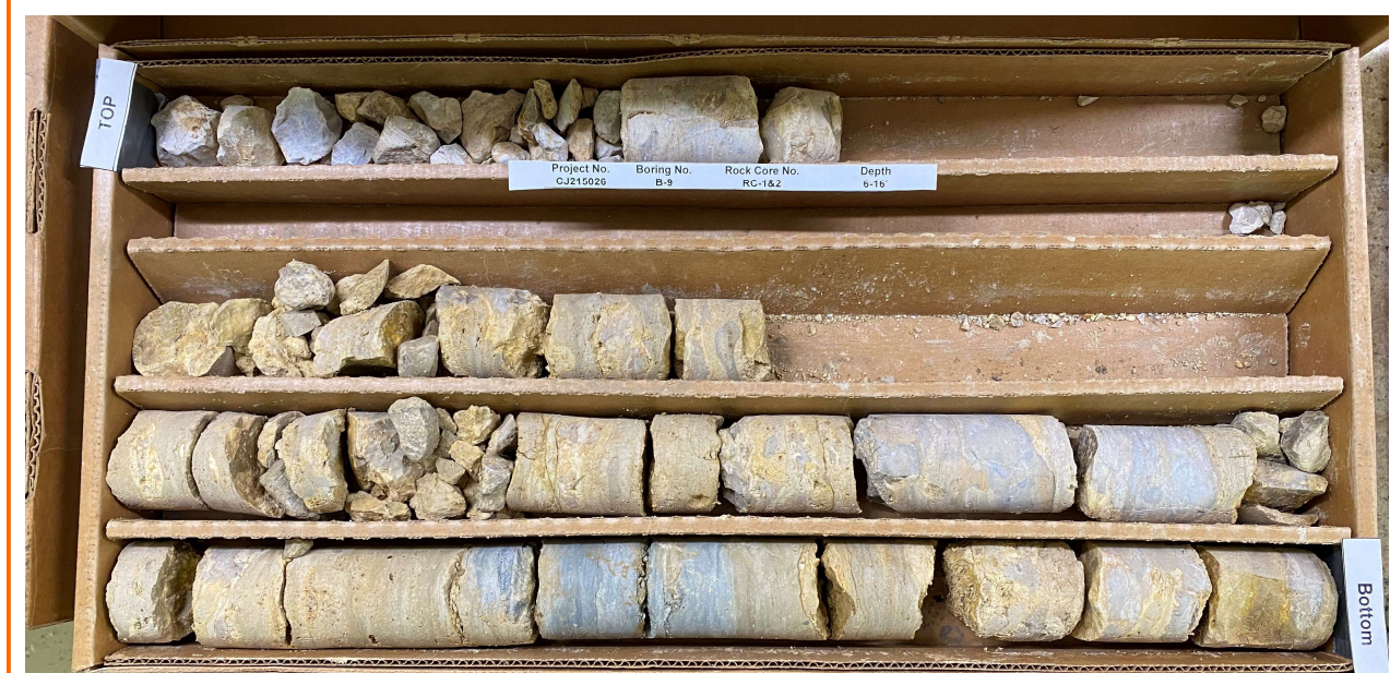
Boring B-9, Rock Core No. RC-1 & 2, Depth 6 to 16 ft
