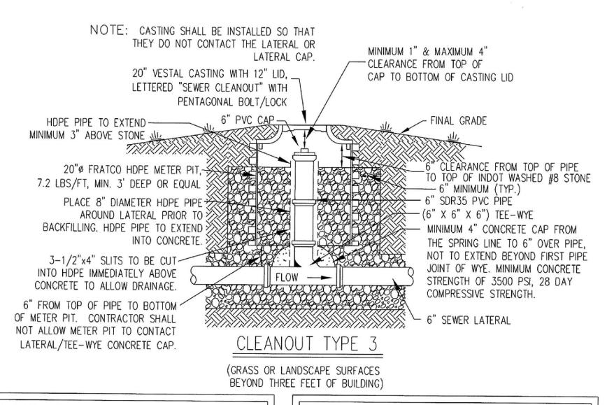
NOTE: TOP OF CASTING OR CLEANOUT CAP SHALL EXTEND 0.20 FEET MINIMUM ABOVE FINISHED GRADE UNLESS CONSTRUCTED WITHIN PEDESTRIAN OR VEHICULAR TRAFFIC WAY. UNLESS APPROVED BY ENGINEER, SANITARY SEWER CASTINGS OR CLEANOUTS MUST NOT BE WITHIN ONE (1) FOOT HORIZONTAL DISTANCE OF ANY PAVED OR CONCRETE SURFACES.
