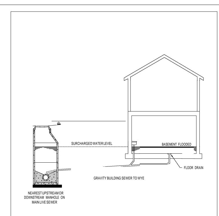
A SANITARY SEWER BUILDING CONNECTION CONSTRUCTED IN THIS SITUATION WILL NOT BE ACCEPTED (SEE THE ACCEPTED SITUATION - FIGURE 1-2)
